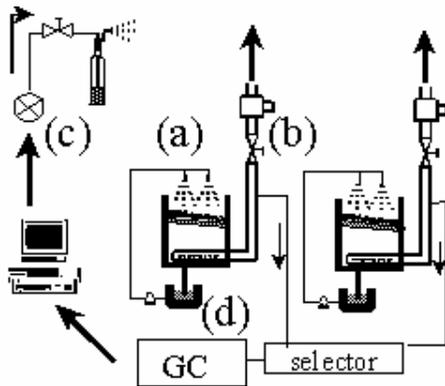
**Figure 1.** Schematic of biofilter apparatus (two biofilters shown). a) misting, b) effluent fan, c) VOC emitter, d) biofilter sump
