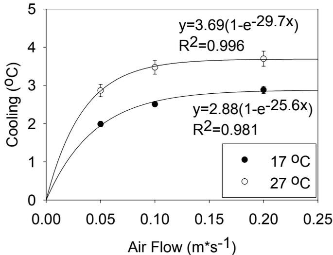
**Figure 4.** Influence of airflow on effluent cooling
