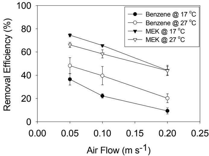
**Figure 2.** Effect of airflow and temperature on biofiltration of MEK and benzene
