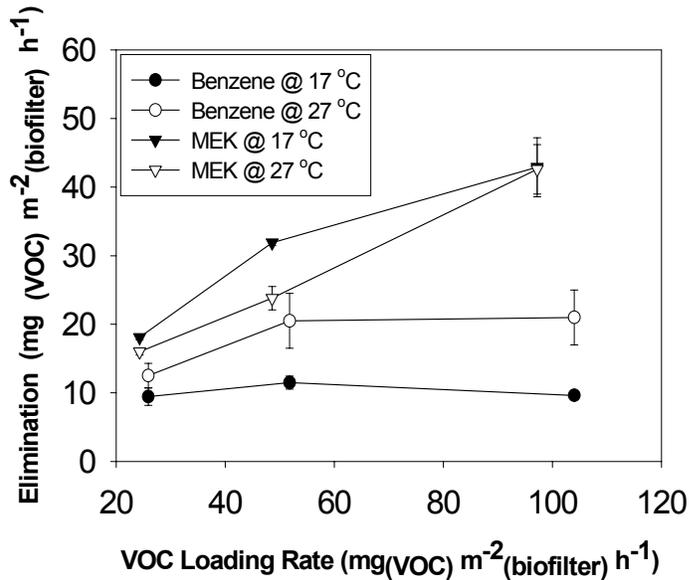
**Figure 3.** Mass VOC loading and elimination rates at 17 and 27 °C
